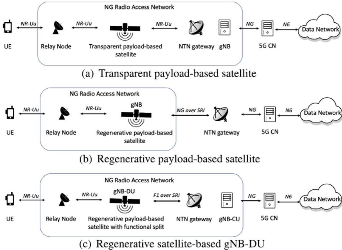
Figure 4-18: Relay-like architecture [90]
