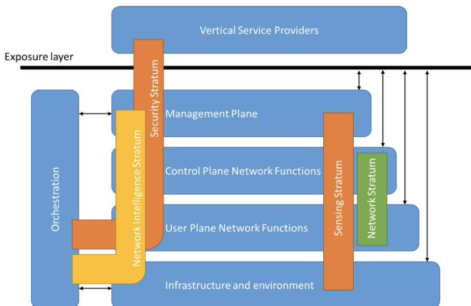
Figure 4-29: Architectural view for 6G by 5G PPP (image reproduced from [112])
