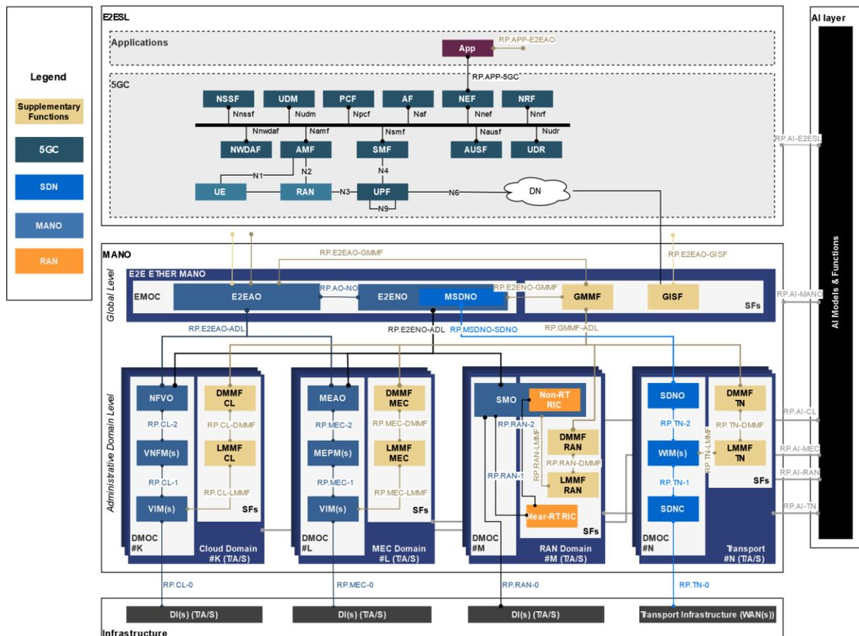
Figure 4-33: Interface map of the ETHER architecture
