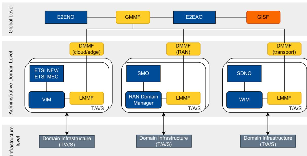
Figure 4-10: Infrastructure mobility management model integrated within ETHER MANO architecture
