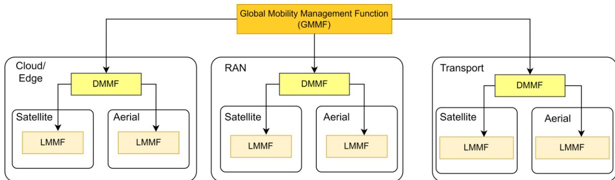
Figure 4-9: Infrastructure mobility management model applied in ETHER 3D Networks
