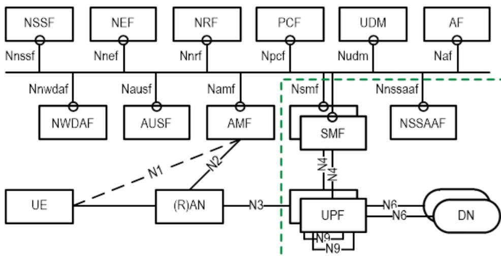
Figure 4-12: Network slicing in 5GS
